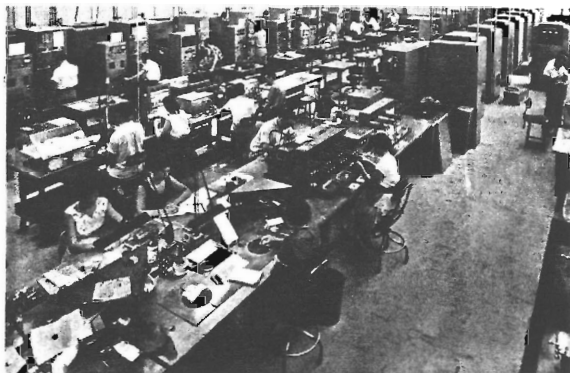
FIG. 3-41. Silicon and germanium crystal growing, using 450-kc r-f generators. (Texas Instruments, Inc.)
