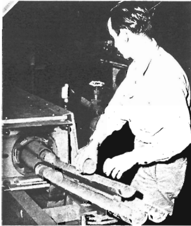
FIG. 3-5. Muffle induction coil heating steel billets for annealing. (Mullins Co.)
