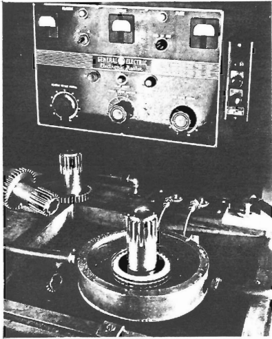
FIG. 3-25. Gear hardening by induction heating. (Cleereman Machine Tool Co.)
