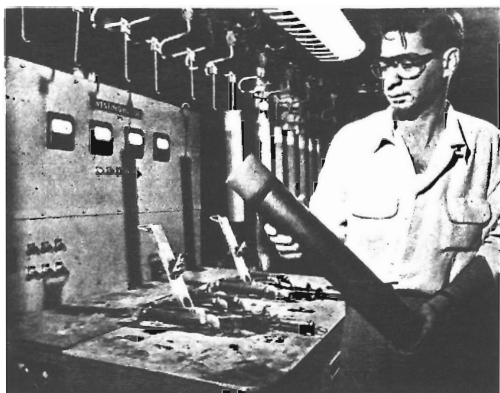
FIG. 3-28. Hardening the inside and sidewalls of steel cartridge cases at motor-generator frequencies. ( Westinghouse Electric Corp. )
