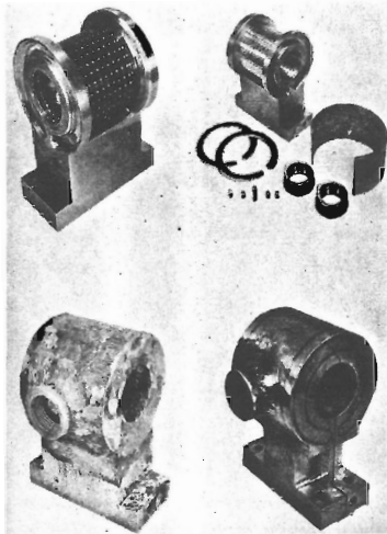
FIG. 4-13. Various stages in the construction of a combined coil-quench block. ( The Ohio Crankshaft Corp. )
