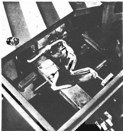
FIG. 3-29. A section blade on a farm mower being hardened by r-f heating.
